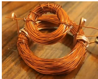
Figure 4. Commutated parallel-excited dc motor. Photo credit: Douyin user @Dover.
